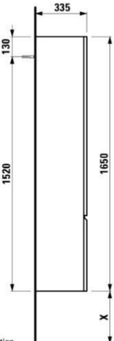
X = The exact height must be set during installation.
