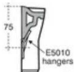
Part section through basin on E5010 hangers
