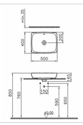
All drawings contain the necessary measurements which are subject to standard tolerances.
